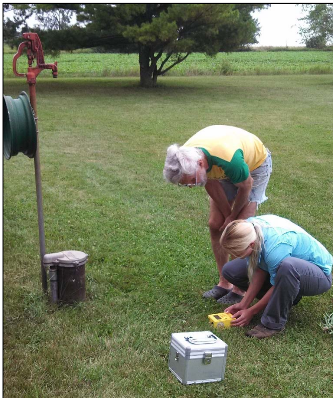
Photos 11 and 12 - The HVSr Passive Seismic instrument shown in the field (left) and up close (right). The three 1-inch metal legs are inserted into the ground to record ambient ground vibrations for bedrock depth data collection. A computer mouse is shown for scale in the photo on the right. Ambient ground vibrations occur due to movement of objects at the ground surface penetrating down into the earth, such as the vibrating roots of a tree blowing in the wind.
