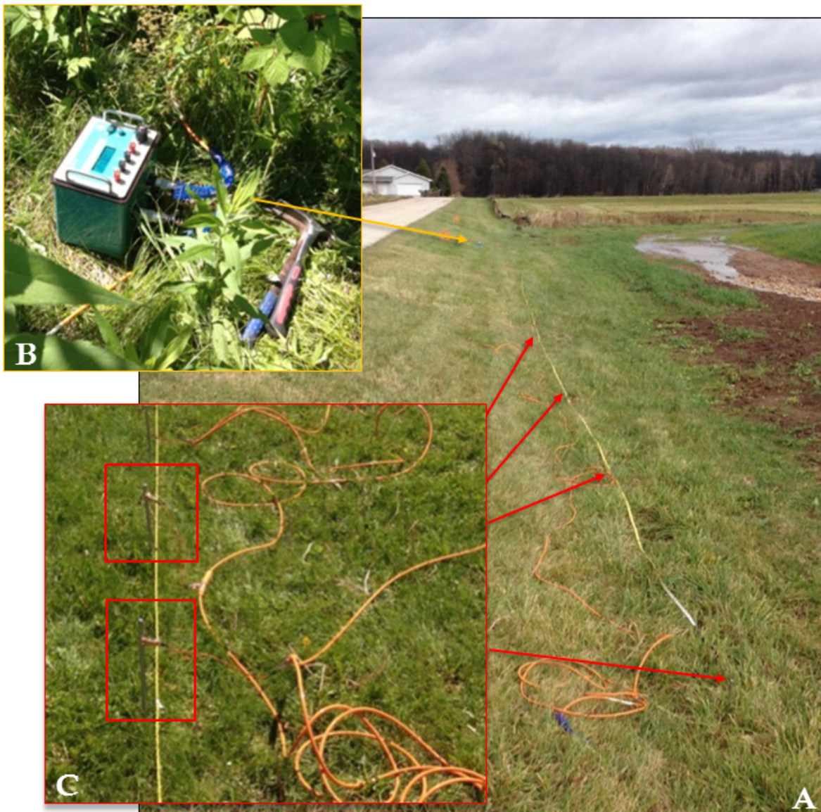
Figure 2 - ERI survey line set-up. A) The survey line is a straight transect. B) The ERI instrument sends a current into the ground through electrodes. C) Electrodes are spaced evenly along the survey line. Two electrodes send the current into the ground, and two electrodes receive the current after it has gone through the subsurface.
