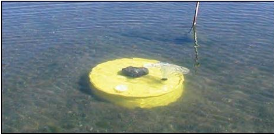
Photo 3 - Seepage meter installed in a lakebed. Clear plastic bag is visible, extending upwards from the top of the yellow cylindrical drum (Rosenberry and LaBaugh, 2008).
