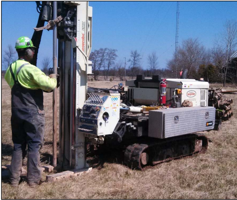
Photos 5 and 6 - Track-mounted Geoprobe drilling rig (left) and subsurface samples collected from Geoprobe drilling (right).
