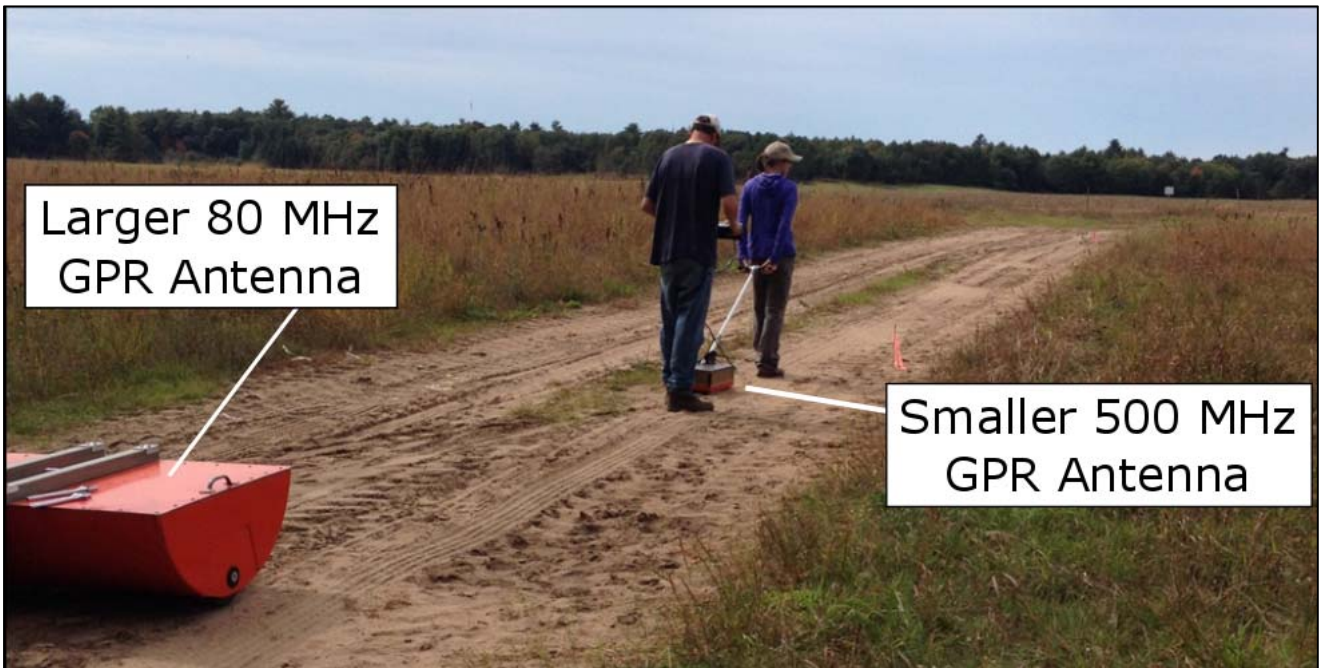
Photo 15 - The smaller 500 MHz Ground Penetrating Radar (GPR) antenna can be used wherever the larger 80 MHz antenna can be used; however, it is smaller and can easily maneuverable in tight areas, such as in a field between rows of corn. The 80 MHz might temporarily flatten taller standing grasses and weeds, but they usually recover after a day. If the 80 MHz were being towed by truck, the minimal damage would be a result of the truck tire tracks.
