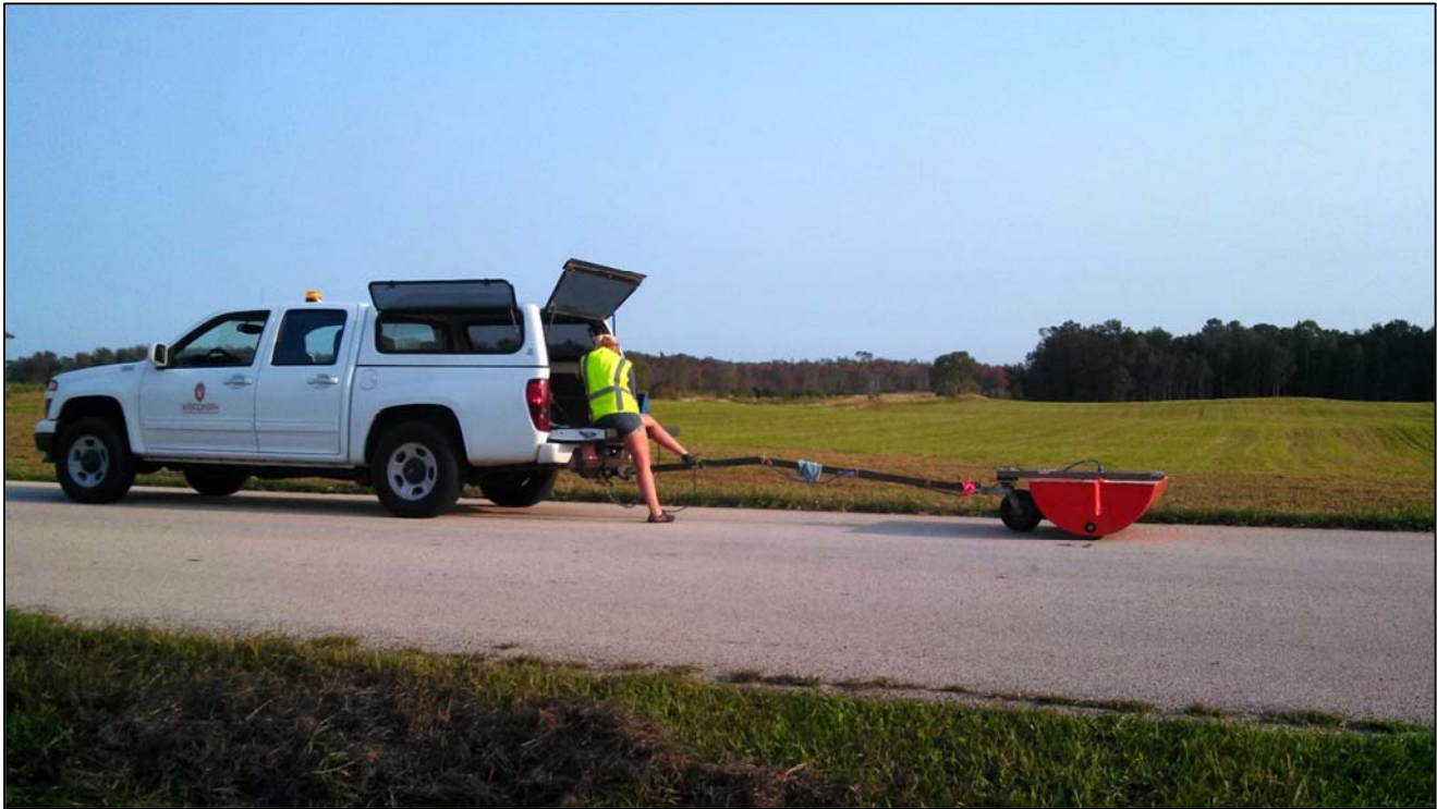
Photo 14 - The 80 MHz Ground Penetrating Radar (GPR) in action on the road. This unit is typically pulled behind a pickup truck along roads or open fields at slow speeds (about 5 mph).
