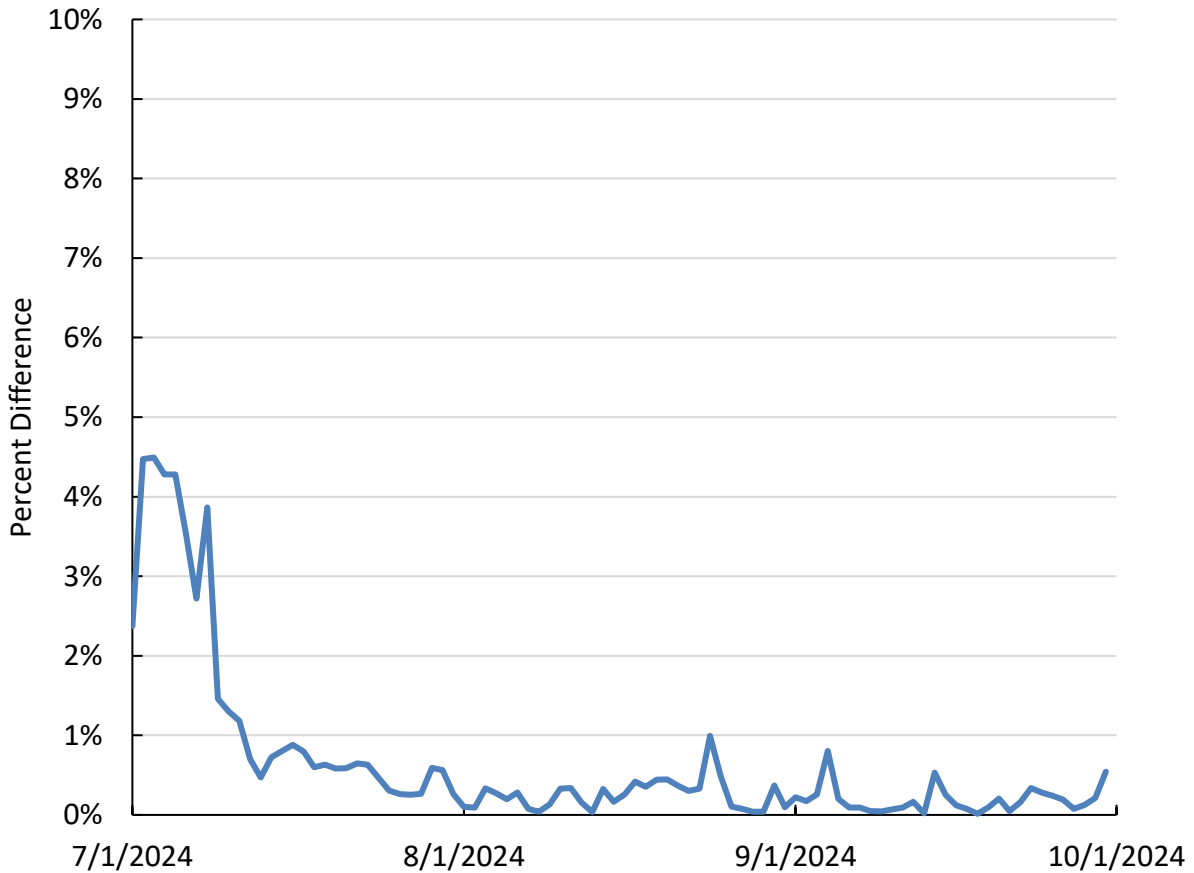
Figure 2. Percent difference between the USGS and CWP daily volume in July through September 2024. A positive value indicates USGS flow measurement is greater than the CWP's measurement.
