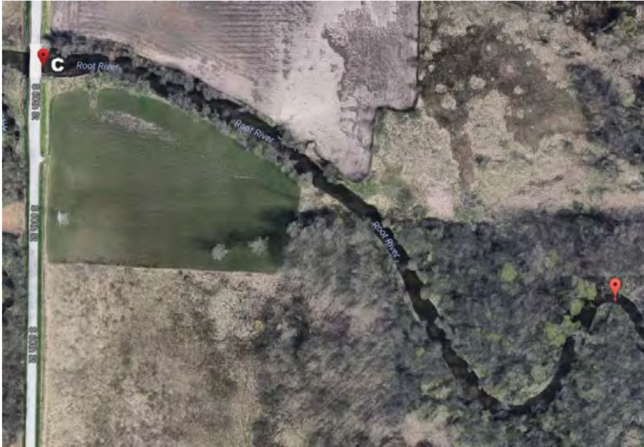
(C) Root River on 60 th Street bridge, at return flow outfall – Biological and habitat sampling reach shall be 35 times the stream width, or approximately 1,995 ft.
