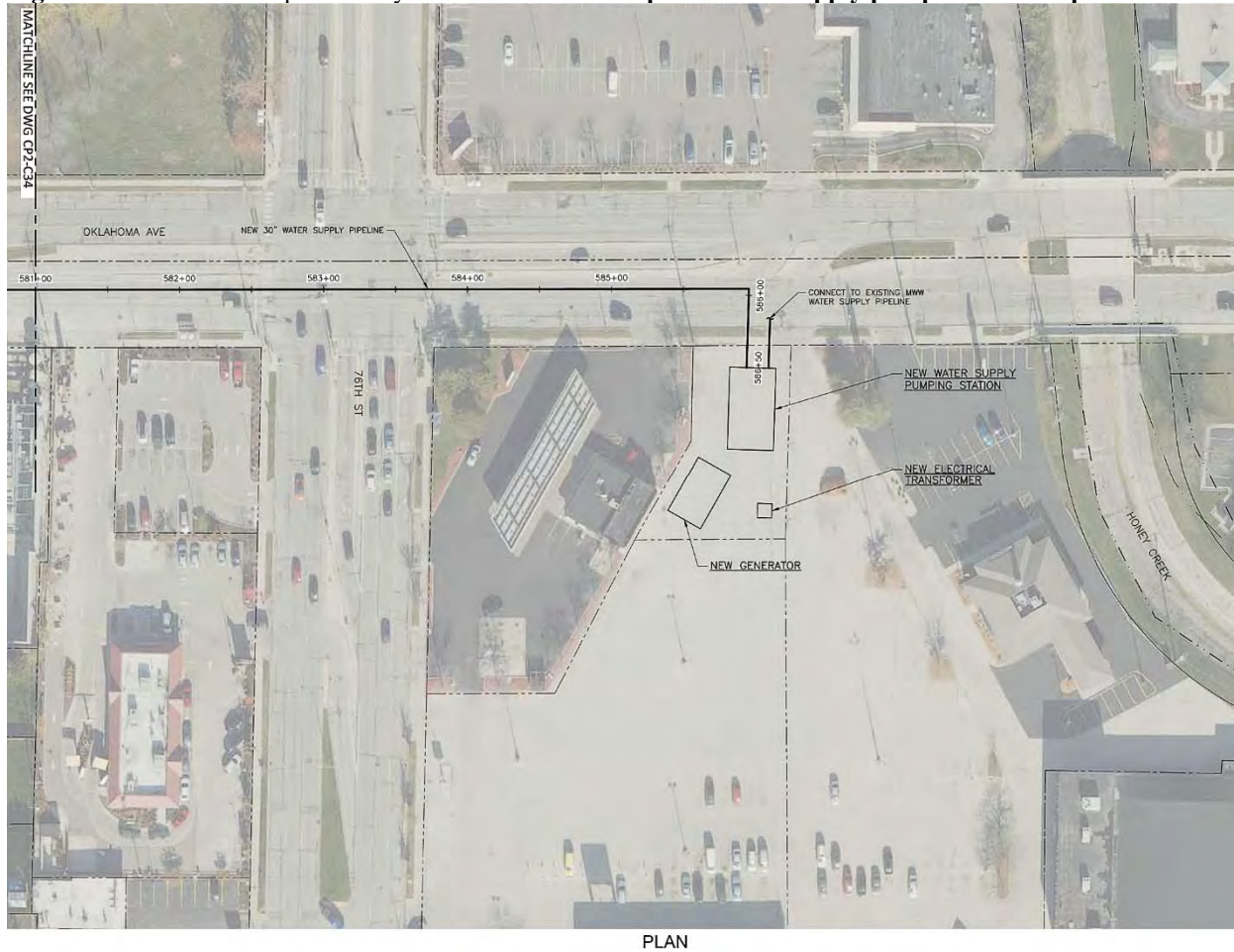
Figure Error! No text of specified style in document.-1. Proposed water supply pump station site plan
