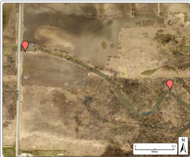
(C) Root River on 60 th Street bridge, at return flow outfall – Biological and habitat sampling reach shall be 35 times the stream width, or approximately 1,995 ft. reach.
