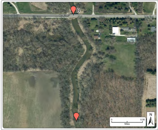
(B) Root River Canal at 7 Mile Road – Biological and habitat sampling reach shall be 35 times the stream width, or approximately 1,050 ft. reach.
