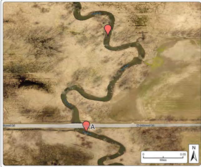
(A) Root River at Oakwood Road – Biological and habitat sampling reach shall be 35 times the stream width, or approximately 1,225 ft. reach.
