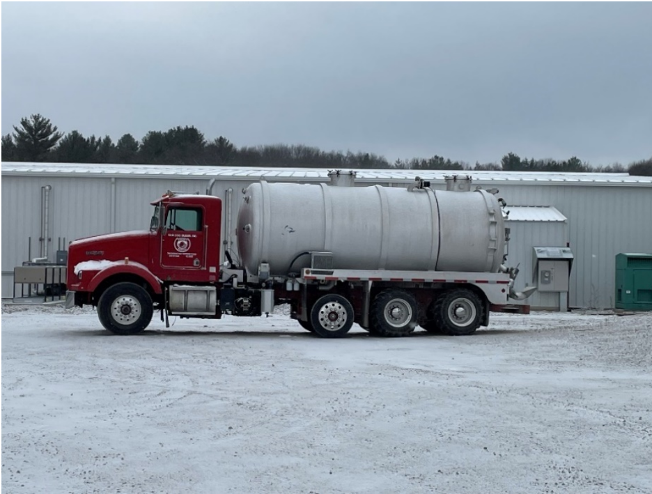
Photo 7: Truck S&R Egg Farms uses for land application of egg wash water.
