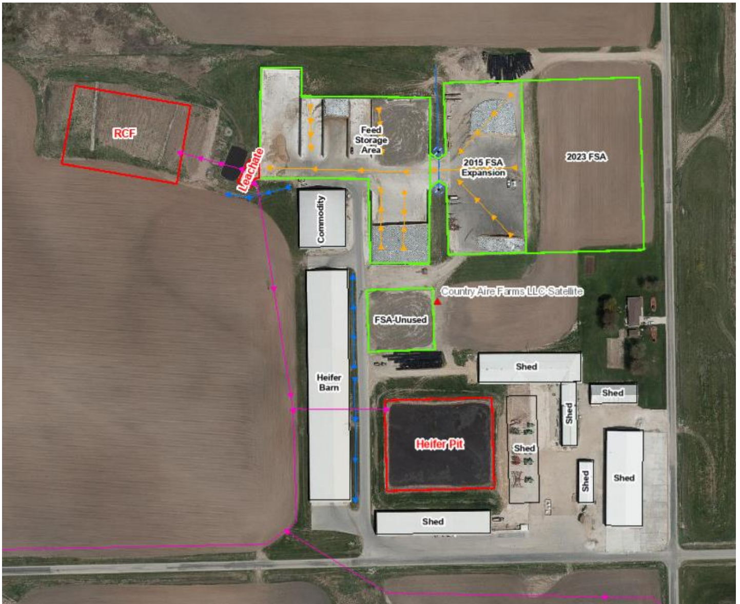
Figure 2. Aerial overview of Country Aire Farms on the north side of Lamers Clancy Road. Blue arrows indicate approximate stormwater flow paths. Yellow arrows indicate approximate contaminated runoff flow paths. Pink arrows indicate manure transfer systems.
