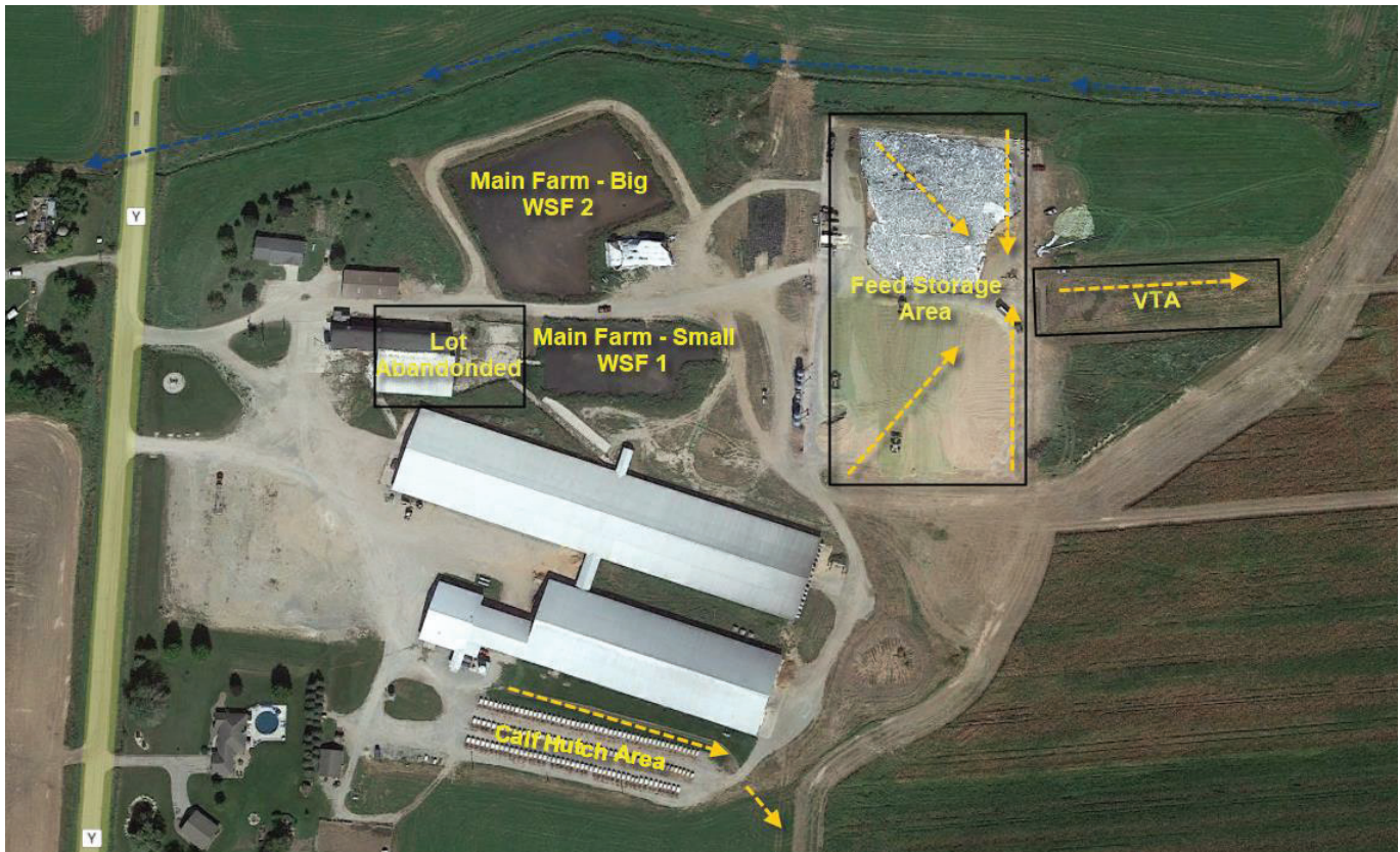
Figure 1. Aerial overview of Vandehei Farms: Main Farm. Yellow arrows indicate flow paths for manure or leachate, blue arrows indicate surface water flow.
