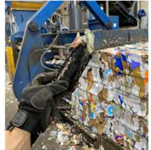
A punctured or bent lithium-ion battery can produce enough heat to melt or ignite materials near the battery, even if the battery itself does not ignite. Photo Credit: Outagamie County Recycling and Solid Waste
