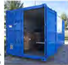
This covered roll-off container provides indoor storage and can be locked for security purposes.
