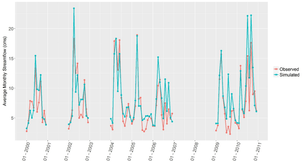
Figure D- 6. Monthly streamflow calibration hydrograph for USGS site 04078500 (Embarrass River near Embarrass, WI).
