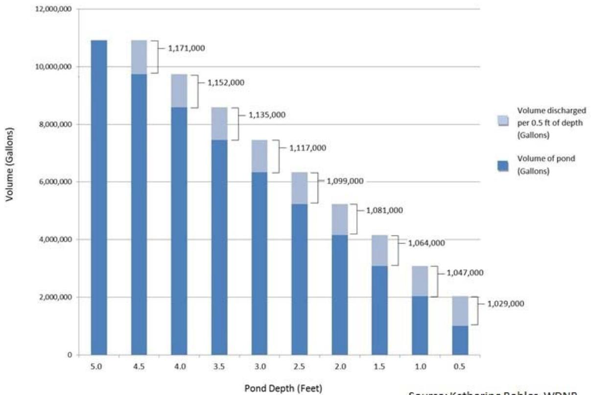
5.4.3 Given data for a fill and draw pond system, calculate the volume of drawdown (gals) required and the time (days) required to achieve drawdown.
