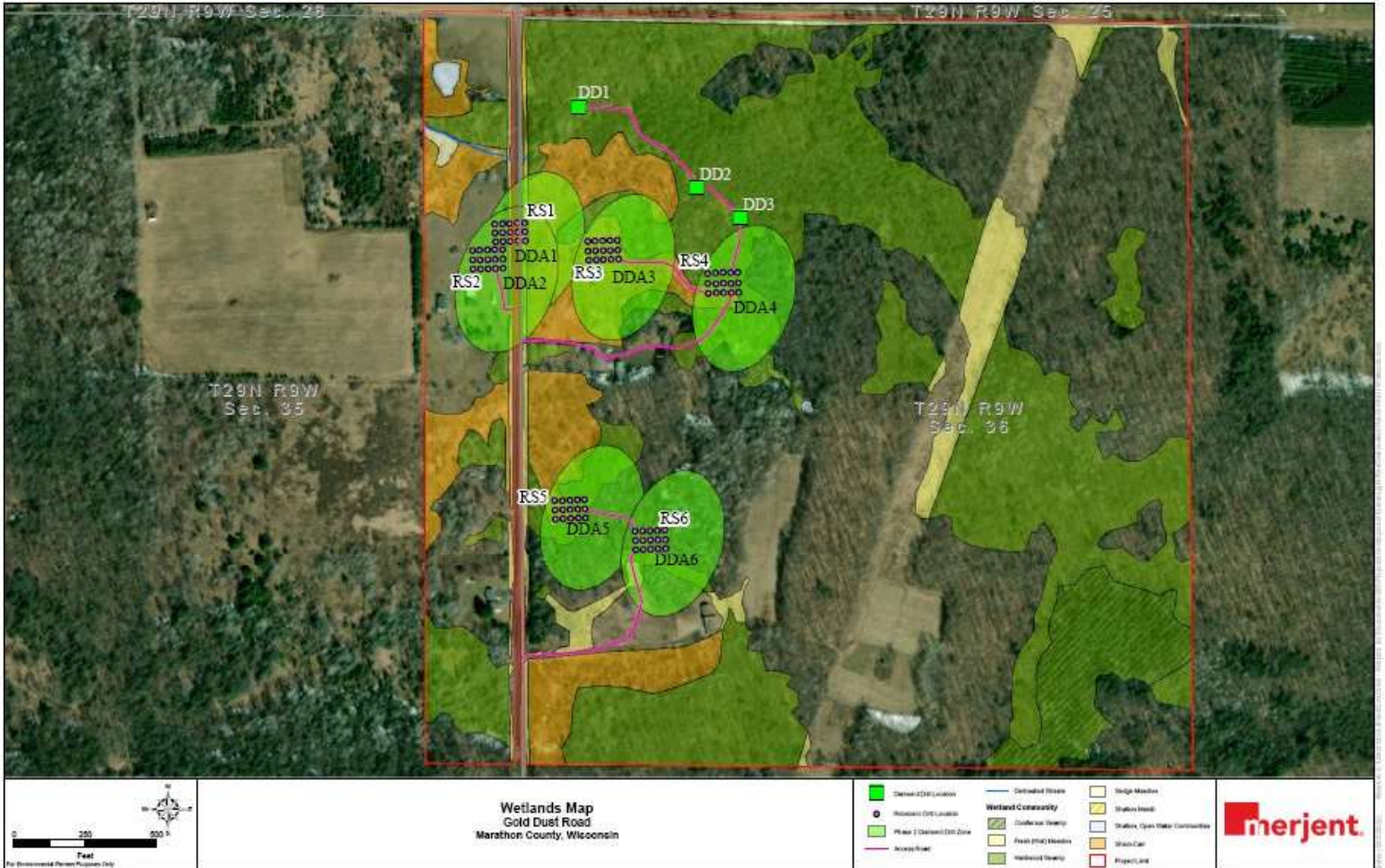
Fig. 4 Wetland map showing diamond drill (DD1-3) sites, roto sonic grid drill sites (RS1-6), potential diamond drill site areas (green areas; DDA1- 6), and access roads/trails. The underlying wetland map is taken from the wetland delineation report prepared for this drilling program and filed with the Wisconsin Department of Natural Resources (WDNR)
