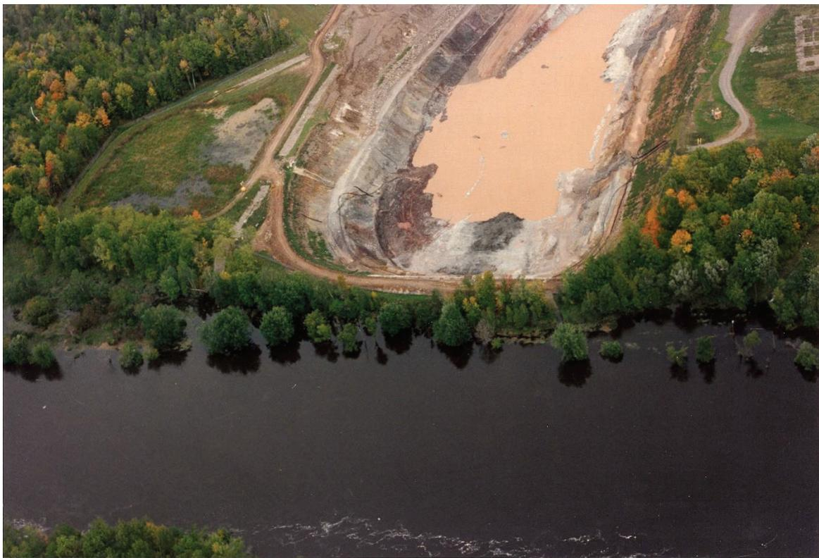
*The Flambeau River came within 20 horizontal feet and 4 vertical feet of spilling into the Flambeau Mine pit in September 1994 during heavy rains, as Rusk County experienced a flood of such magnitude that it exceeded a hundred-year event. This photo was taken the day after the river crested (Photo by Bob Olsgard of Sarona, WI, September 17, 1994).*
