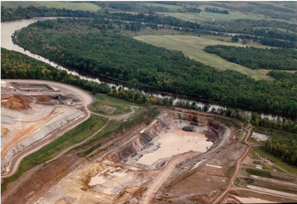
*Aerial view of the Flambeau Mine shows the pit with accumulated precipitation and groundwater in the bottom and its close proximity to the Flambeau River. To the left is the high-sulfur waste rock stockpile, ore crushing area, rail spur, and an engineered runoff pond (Photo by Bob Olsgard of Sarona, WI, September 17, 1994).*
