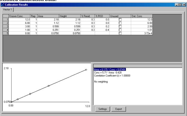
The calibration series was 1, 3, 6, and 12 mg/L NH<sub>3</sub>-N, including a reagent blank. The standards for the distilled calibration were carried through the same distillation as the samples, LCS and reagent blanks.
