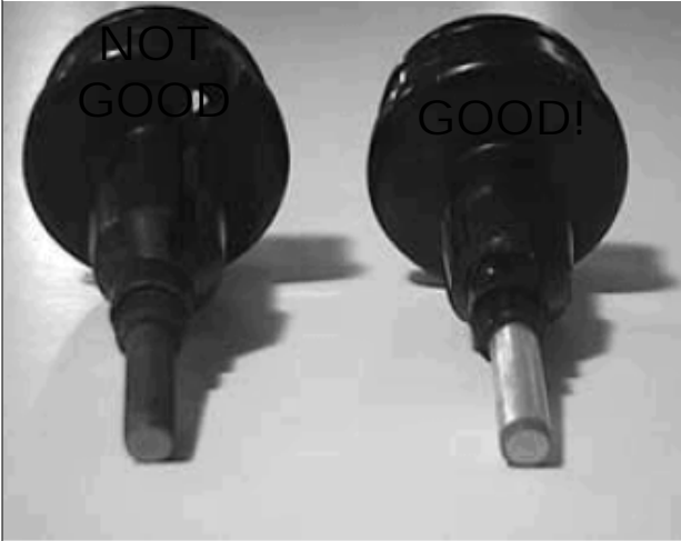
Figure 1. On the right is a properly prepared cathode and anode. Note the light silver appearance of the anode and matte finish of the gold cathode.
