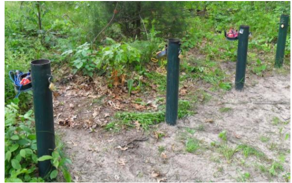
Nested piezometers installed for monitoring groundwater levels and sampling for groundwater contaminants near Spring Green. Photo: Blake Russo-Nixon.
