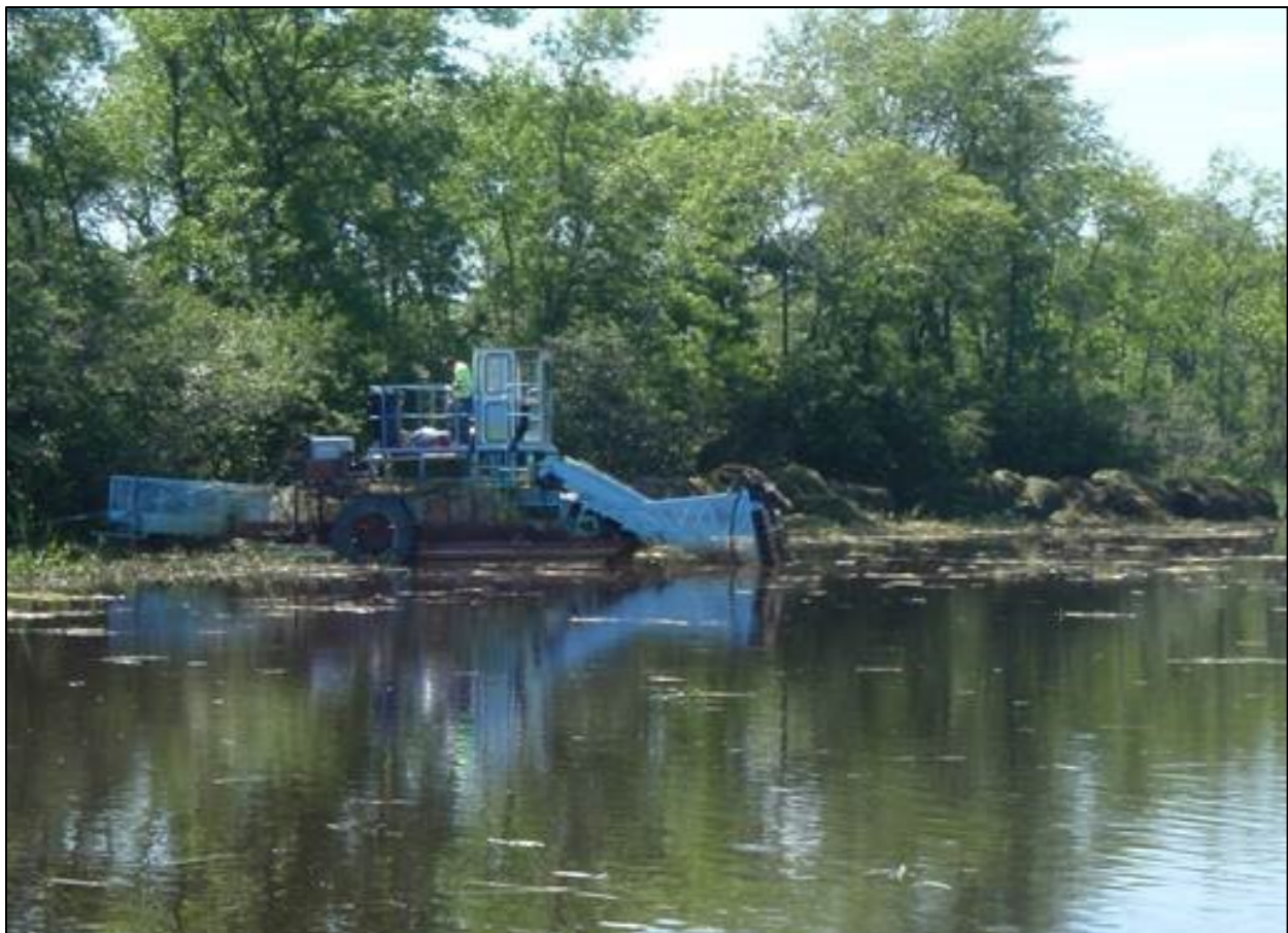
Figure 18. Fond du Lac Band of Lake Superior Chippewa personnel operate a weed harvester to reduce vegetation density in the SLRE (image source: 1854 Treaty Authority).
