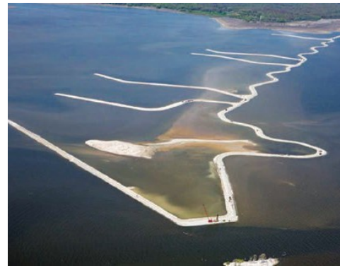
The Cat Island chain framework was completed in 2013. Clean dredged material will be beneficially re-used as fill for the next 20-30 years.
