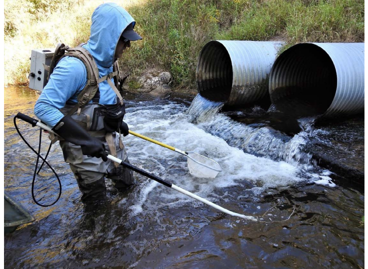
Baseline fish sampling prior to replacing perched culverts in Little Cedar Creek at Sweeter Road to restore fish passage for native Brook Trout. Source: NOAA
