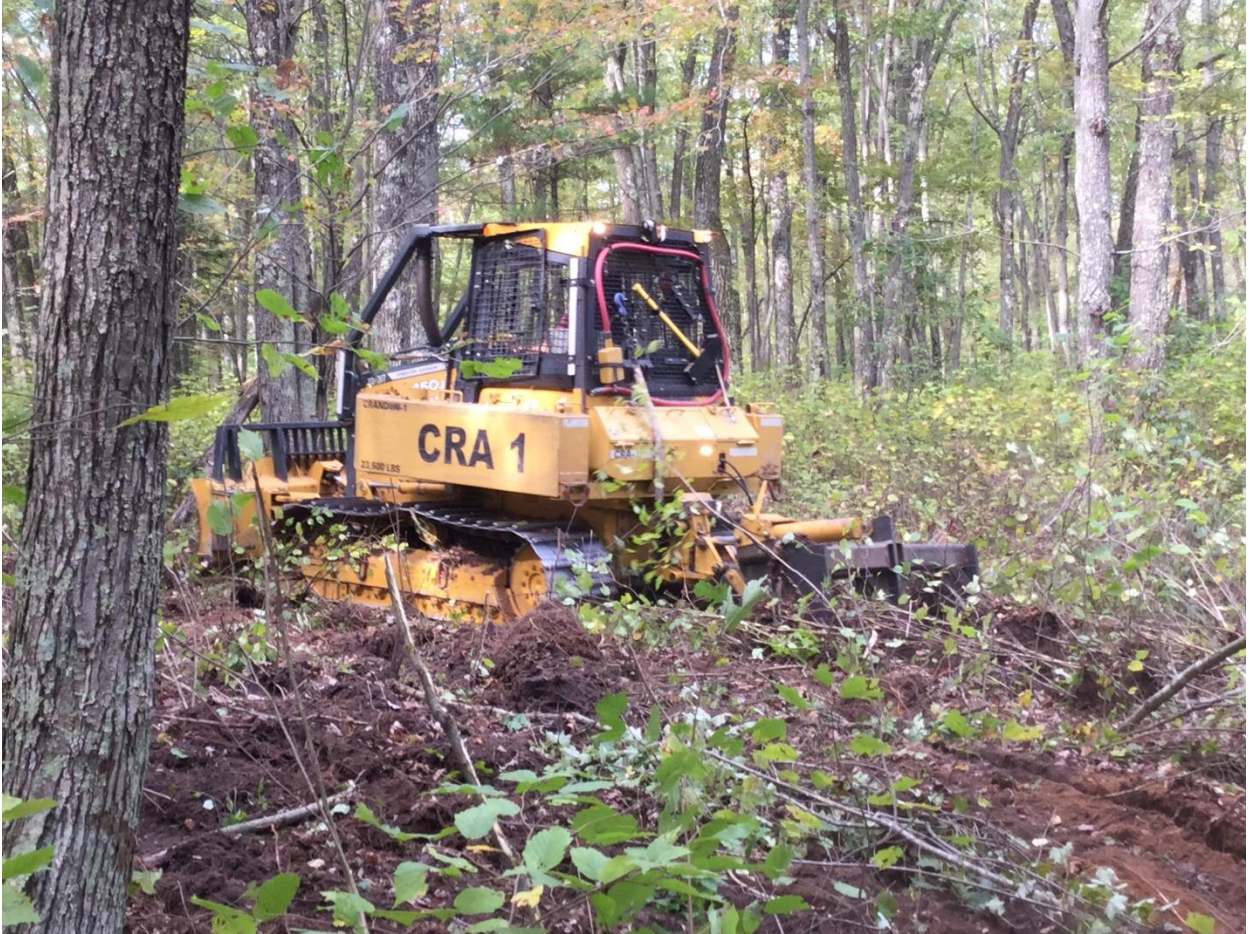
Photo 2 – Headson scarifier in operation
