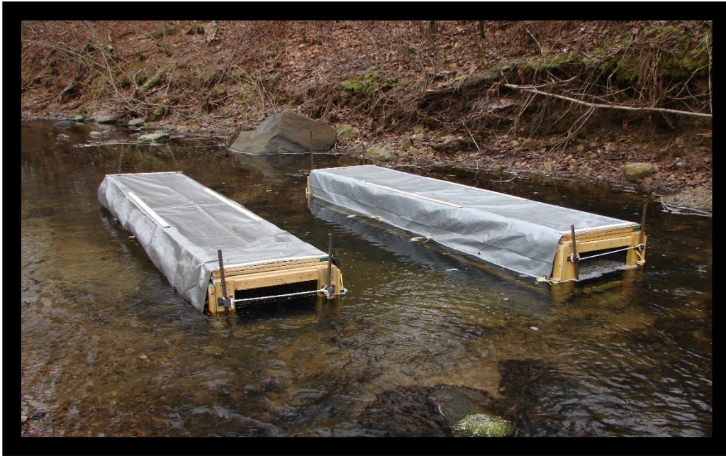
Figure 1. In-stream holding pens for adult brook trout in the South Fork Hay River, Barron County, Wisconsin.
