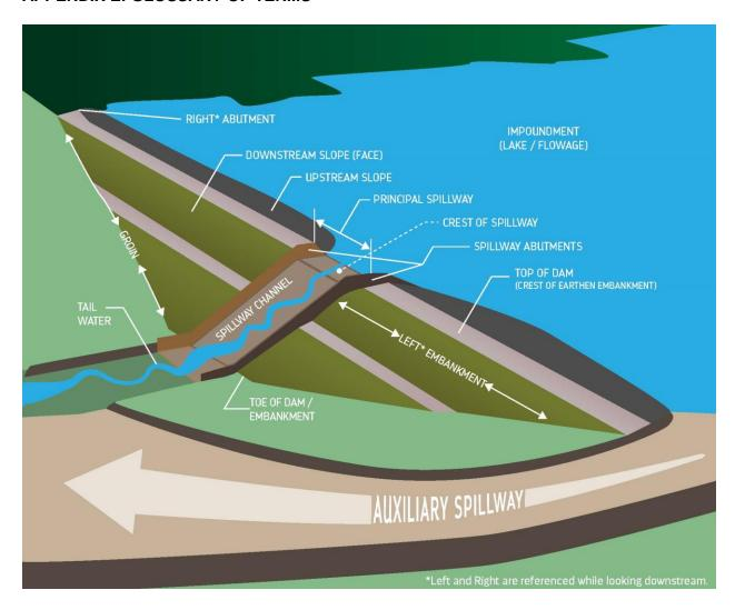
**Abutment** – That part of the valley side or concrete walls against which the dam is constructed. An artificial abutment is sometimes constructed where there is no suitable natural abutment. The wall between a spillway or gate structure and the embankment can also be referred to as an abutment. (Also see Spillway Abutment)
