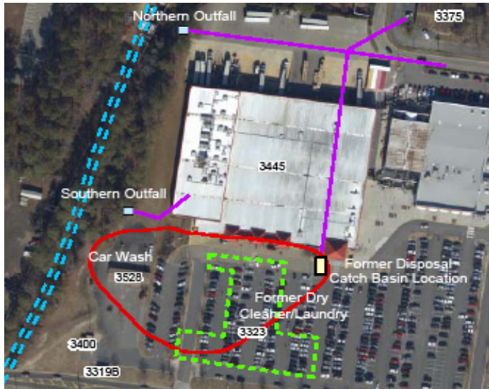
Legend - Groundwater Plume Treatment Area - Former Building Locations - Freshwater Canal - Former Storm Water Line - Outfall Location - Former Disposal Catch Basin Location Note: Storm Sewer was removed during construction of the commissary (1987 - 1992).
