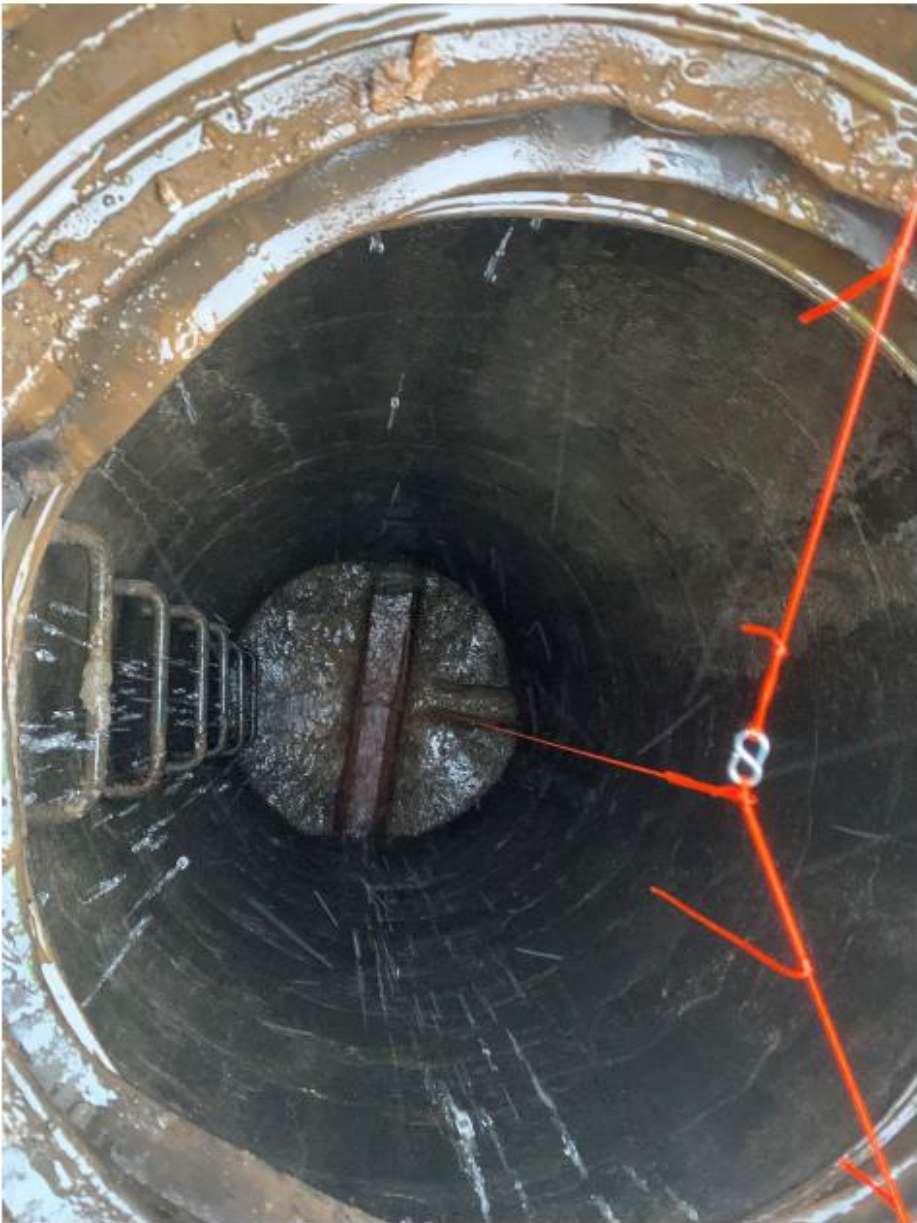
Photo 2: Deployed Beacon sampler hanging in a sanitary manhole structure. September 27, 2023.
