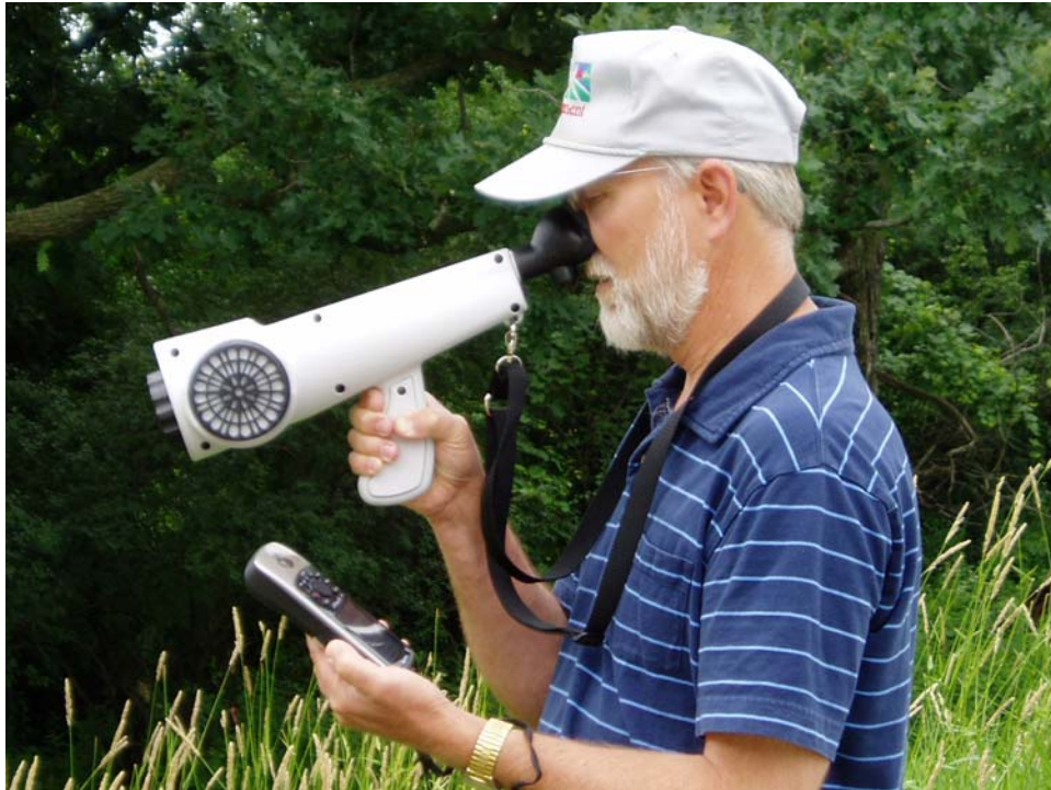
Figure C Using a Nasal Ranger™ and GPS Unit to Take an Odor Measurement in the Field
