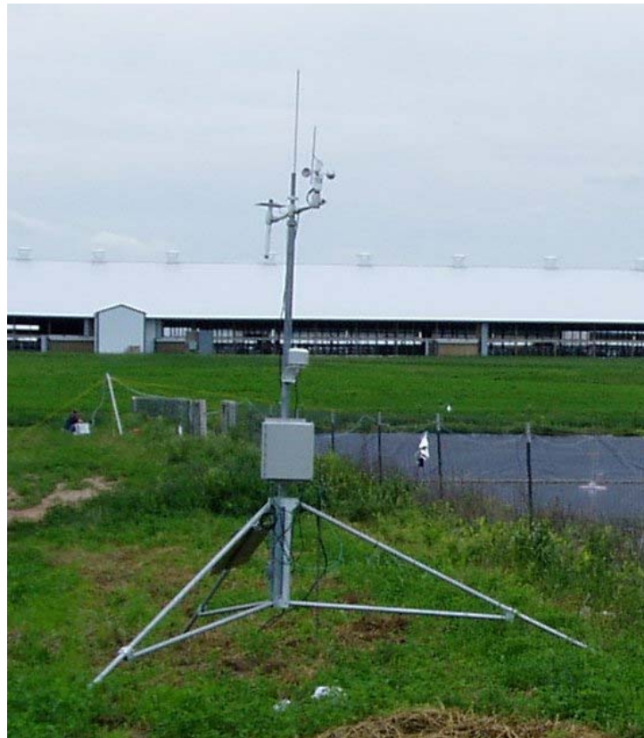
Figure D Solar Powered Meteorological Station
