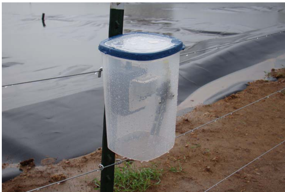
Figure E Sampling Equipment Weather Shelter
