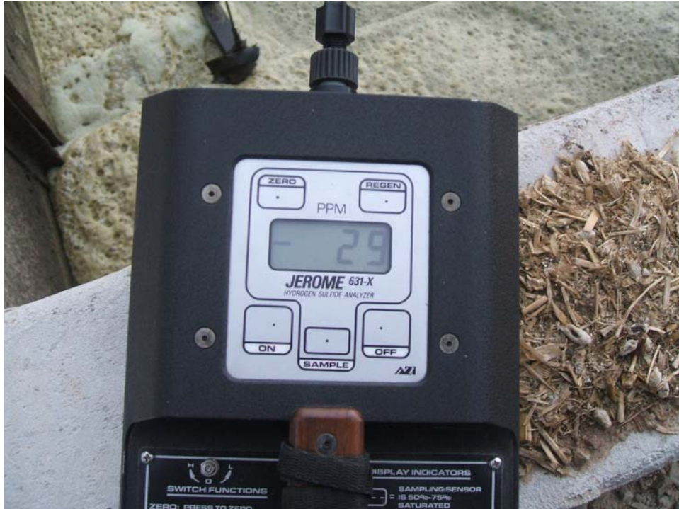
Figure B Jerome Hydrogen Sulfide Meter
